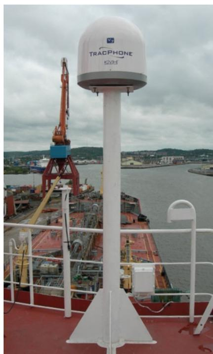
A TracPhone V7 satellite communications antenna allows the Master of the M/T *Primula* to stay in touch with colleagues on shore from any location aboard the vessel.
